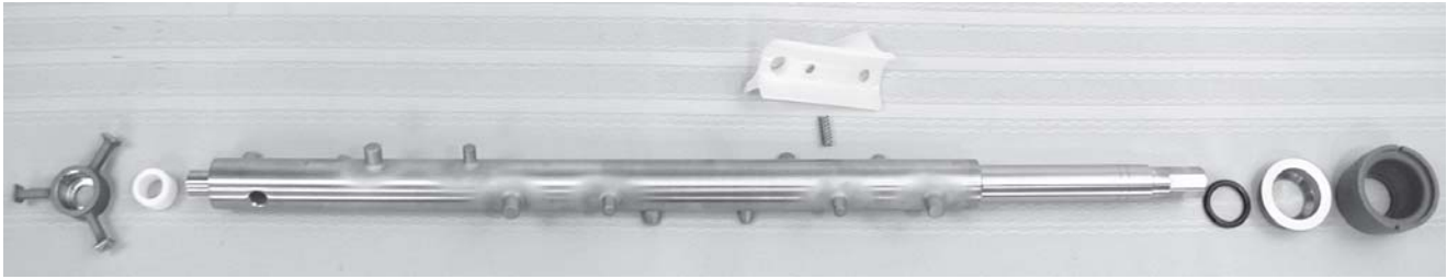
Figure 13. Auger with Rubber Rear Seal
