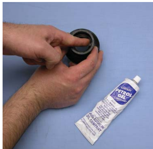
Figure 3-5 Lubricate Rear Seal
