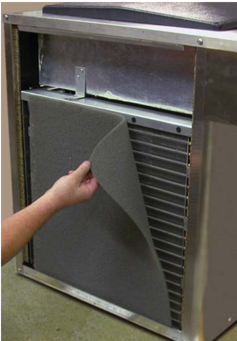
Figure 4-4 F112 Condenser Filter Removal
