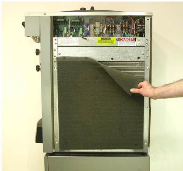
Figure 4-5 Condenser Filter Removal
