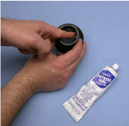
Figure 3-6 Lubricate Rear Seal
