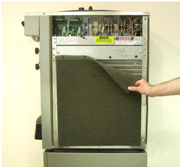
Figure 4-5 Condenser Filter Removal
