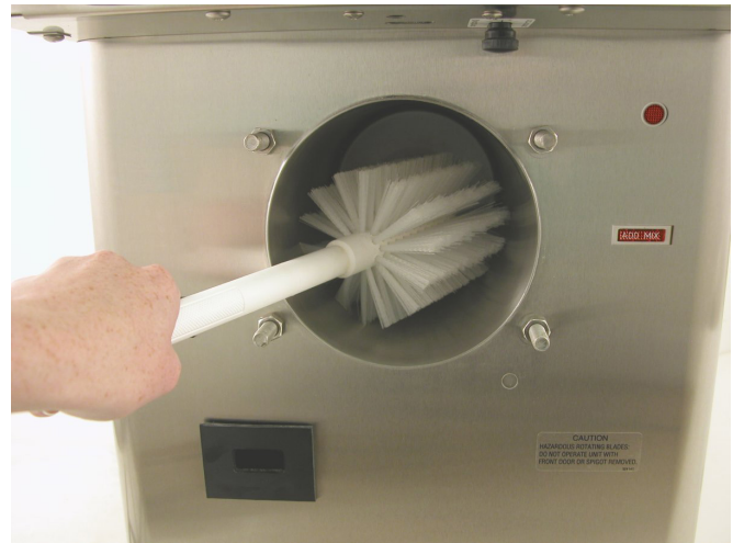
Figure 3-7 Cleaning Freezing Cylinder
