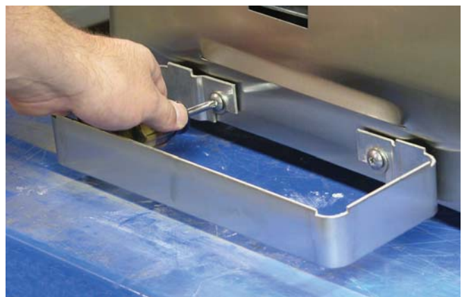
Figure 2-3 Drip Tray Bracket
