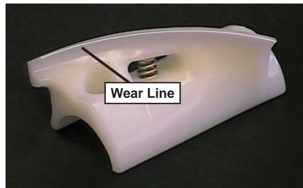
Figure 3-3 Auger Flight Wear
