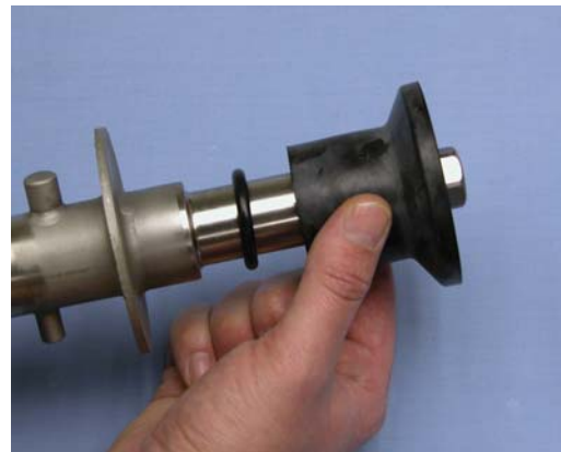
Figure 3-6 Rear Seal Assembly
