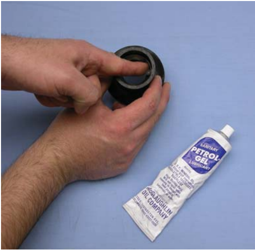
Figure 3-8 Lubricate Rear Seal
