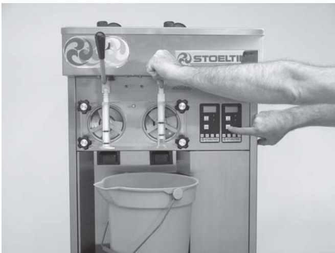
Figure 13. Spigot Opened and Solution Draining
