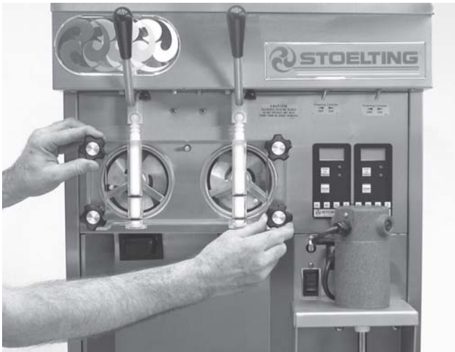
Figure 20. Removing Front Door
