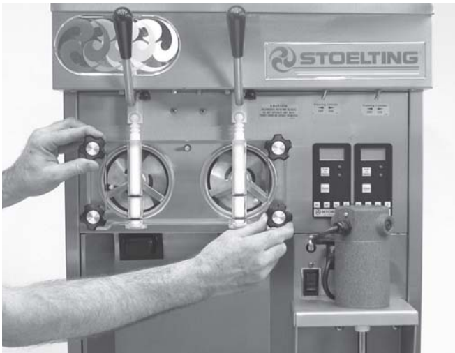
Figure 20. Removing Front Door
