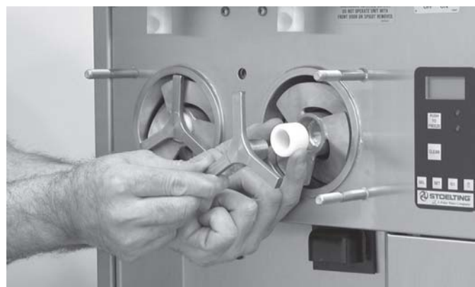
Figure 23. Removing Auger Supports
