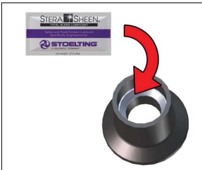
Figure 3-6 Lubricate Rear Seal
