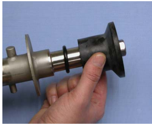
Figure 3-5 Rear Seal Assembly
