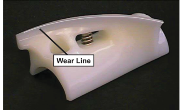
Auger Flight Wear
