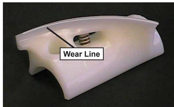
Figure 3-3 Auger Flight Wear
