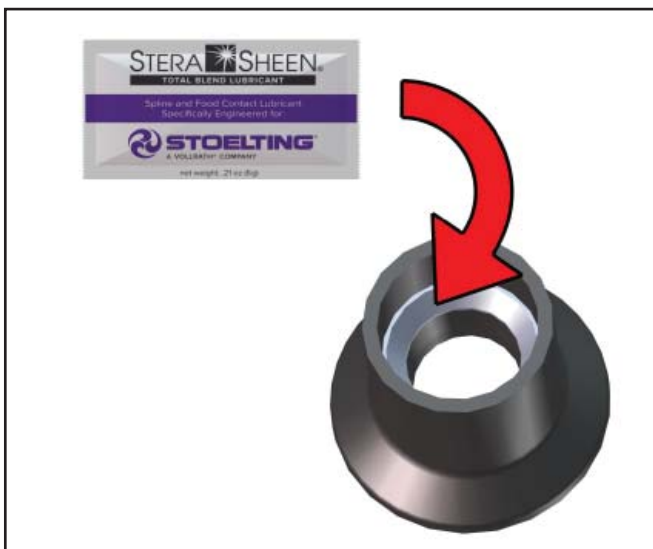
Figure 3-6 Lubricate Rear Seal
