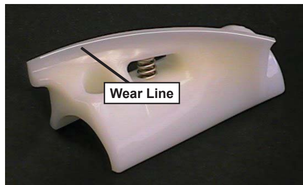
Figure 3-3 Auger Flight Wear
