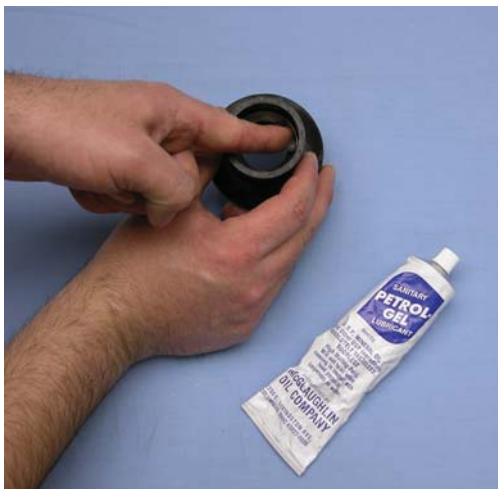
Figure 3-6 Lubricate Rear Seal
