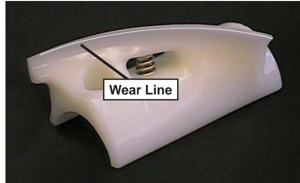
Figure 3-3 Auger Flight Wear
