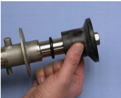
Figure 3-5 Rear Seal Assembly
