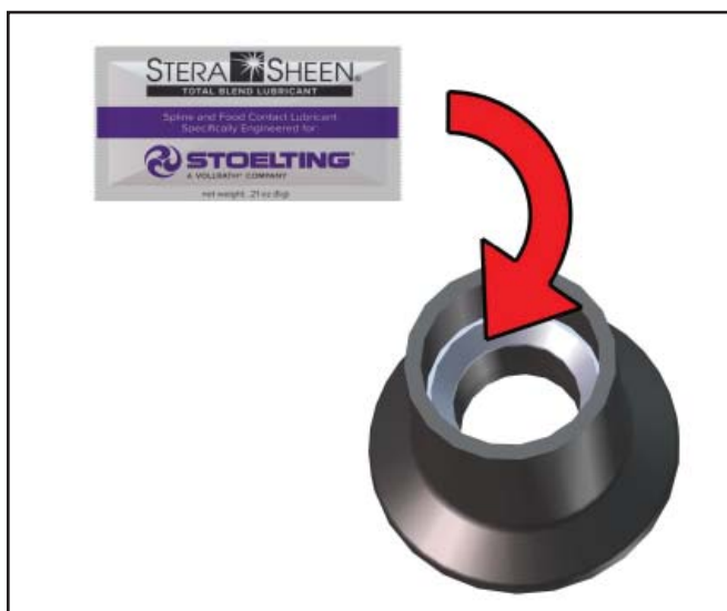
Figure 3-6 Lubricate Rear Seal
