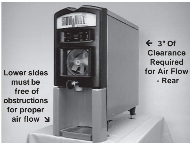
Figure 16. Clearance for Air Flow
