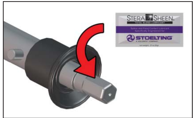
Figure 3-6 Lubricate Hex End of Auger
