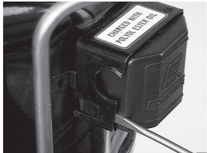
Figure 11. Compressor Terminal Cover Removal
