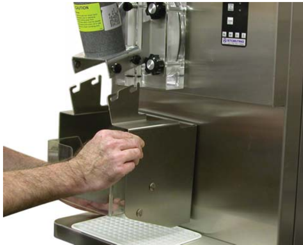
Figure 3-3 Removing Splash Shield Bracket
