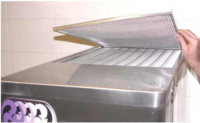
Figure 4-4 Removing Condenser Filter
