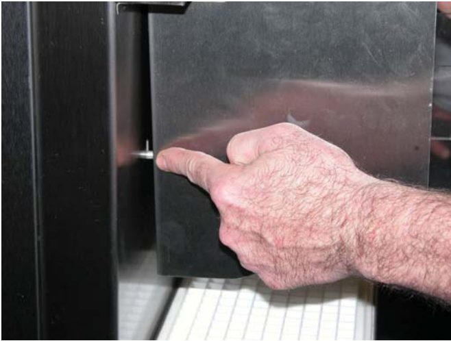
Figure 3-7 Blender Shroud Pin Alignment
