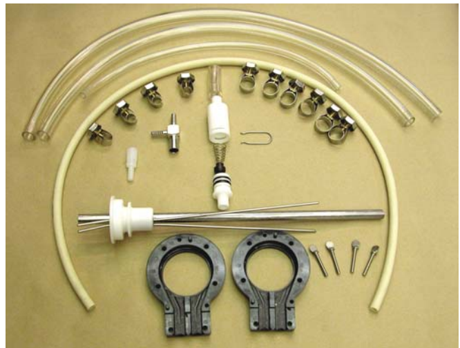
Figure 3-11 Mix Pump Removable Parts
