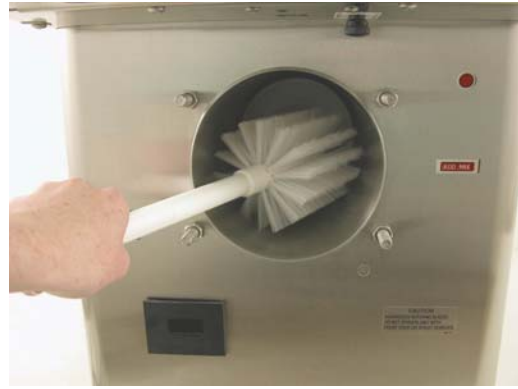
Figure 3-8 Brush Freezing Cylinder
