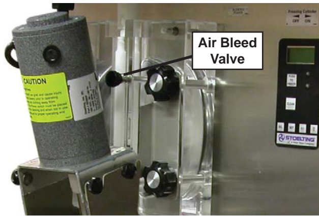
Figure 3-8 Air Bleed Valve
