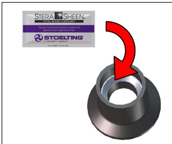
Figure 3-6 Lubricate Rear Seal
