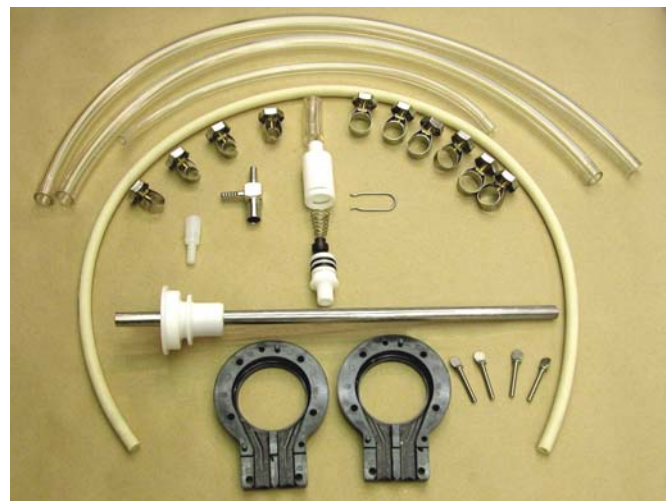
Figure 3-10 Mix Pump Removable Parts
