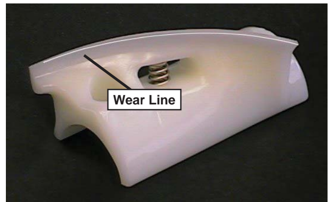
Figure 3-3 Auger Flight Wear
