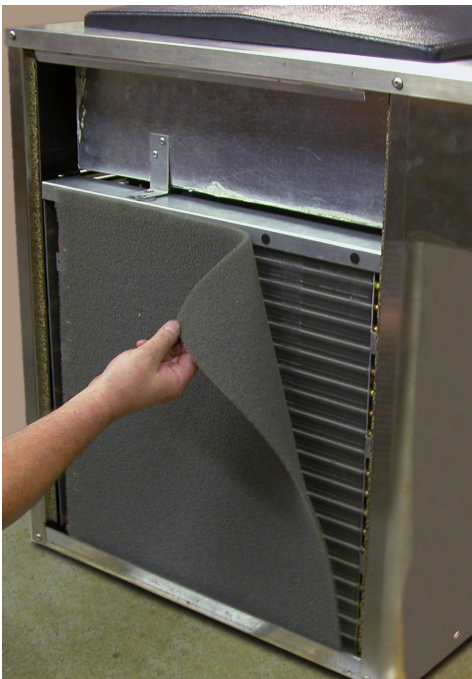
Figure 3-11 F112 Condenser Filter Removal
