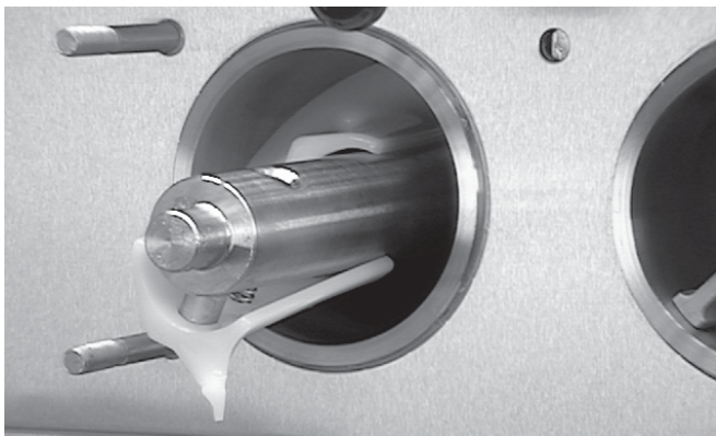
Figure 19. Auger Flight Removal
