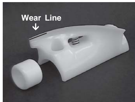
Figure 17. Auger Flight Wear & Front Auger Support Bushing Wear
