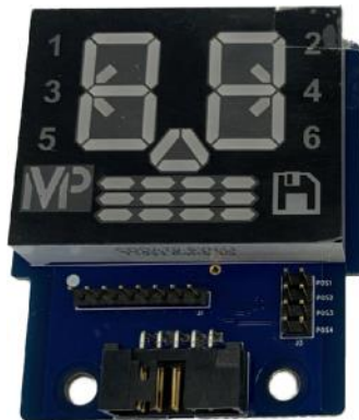
2.3523 —Digital Shot Timer Control Board with LED Digits, (Mounting Hardware and Cover Not Included)
