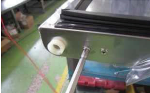
F. Disassemble stopper plate, then tight screws.
