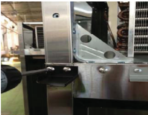
C-1. Disassemble the top hinge (left).
