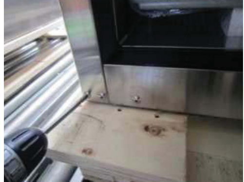
C-2. Disassemble bottom hinge (left).
