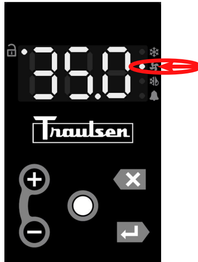
Fig. 4.4a ONLY FAN ICON ILLUMINATES WITH OFF-CYCLE DEFROST
