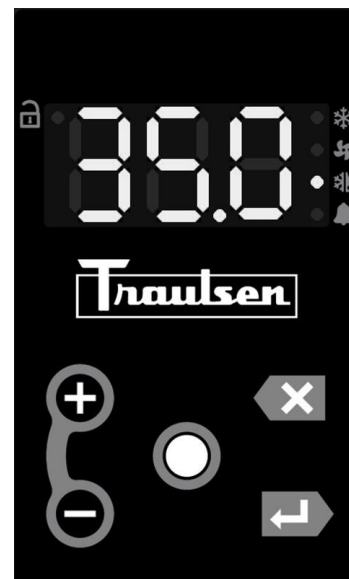
Fig. 6B.15.2a DISPLAY DURING ELECTRIC DEFROST
