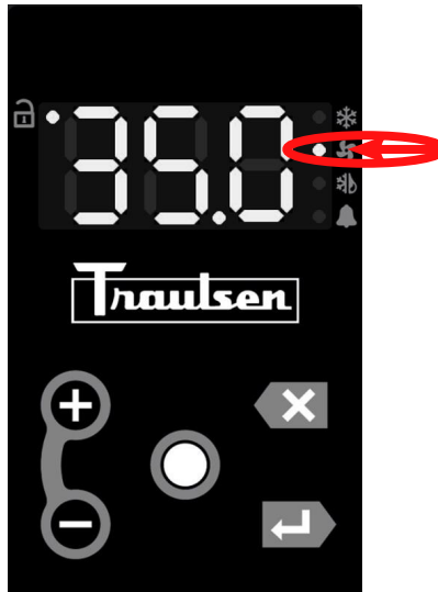
Fig. 4.4a ONLY Fan Icon Illuminates with Off-cycle Defrost
