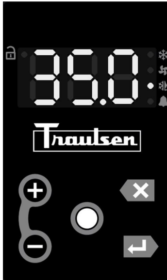
Fig. 6B.12.2b Display During Electric Defrost
