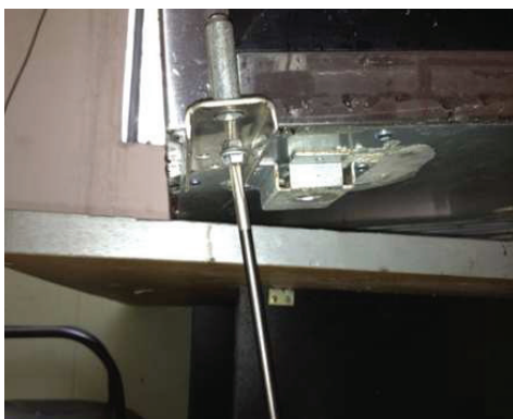
5) Screw the screws located on the bottom left hand hinge.
