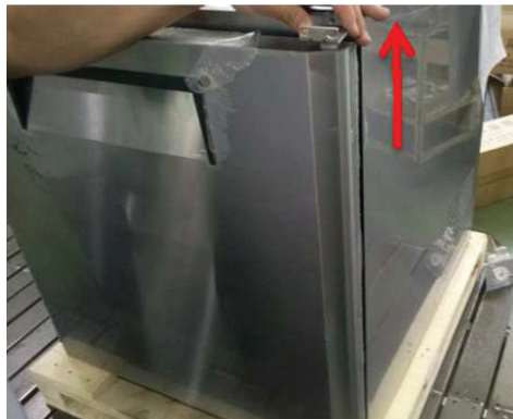
2) Remove the top hinge from the unit.
