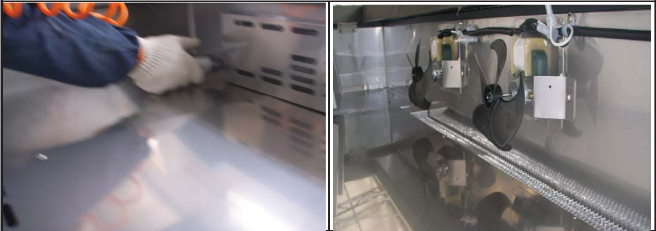
B. Disassemble the evaporator duct
