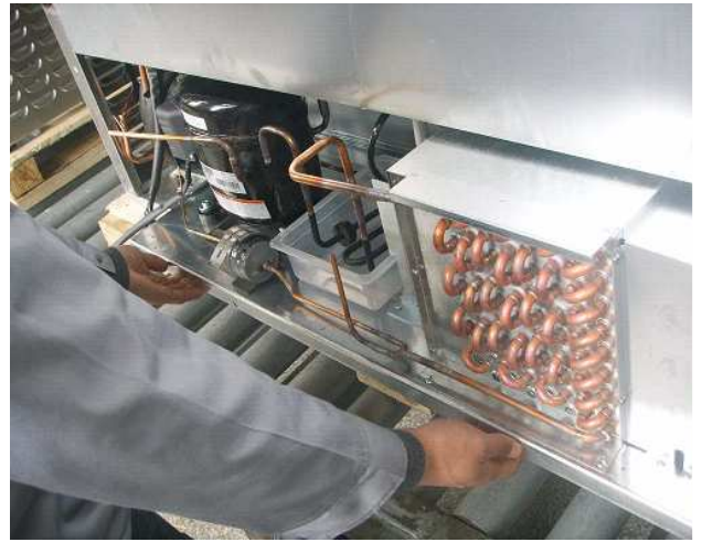
Pull out the condensing unit
