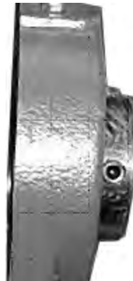
Figure 176. Loosen set screws
