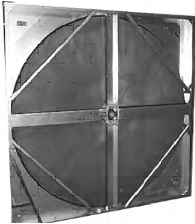
Figure 178. Install bearing mounting bolts
