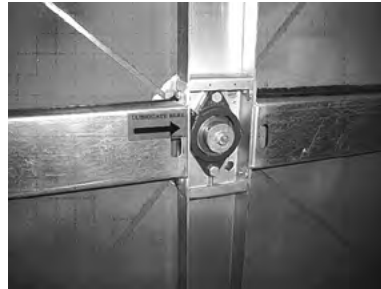
Figure 177. Remove bolts securing bearing
