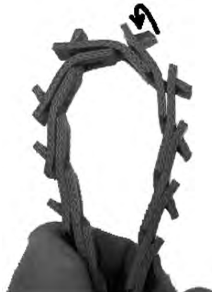
Figure 181. Hold belt with tabs facing outward
