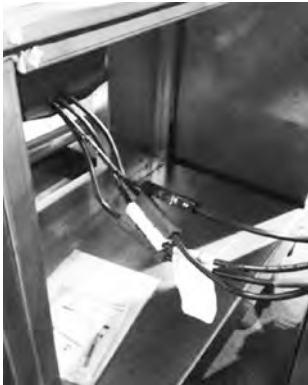
Figure 37. Horizontal section-to-section high voltage quick connects
