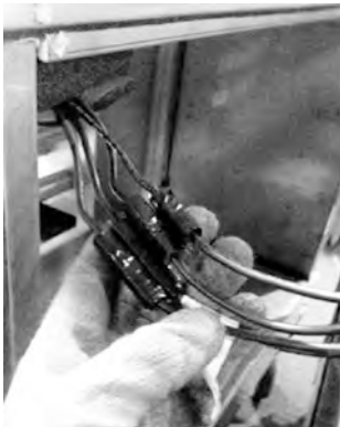
Figure 38. Horizontal section-to-section high voltage quick connects
