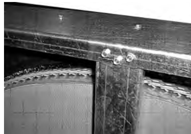
Figure 168. Remove post mounting screws
