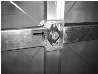
Figure 175. Remove bolt and washer from shaft
