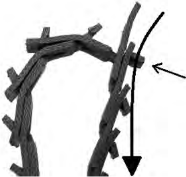
Figure 182. Twist and push through links
