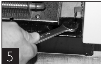
Images 4-6, removing skid from bottom of cabinet.
