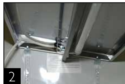
Shelf clips are installed with the front clip lower than the rear clip. This will allow the shelf to tilt forward.
