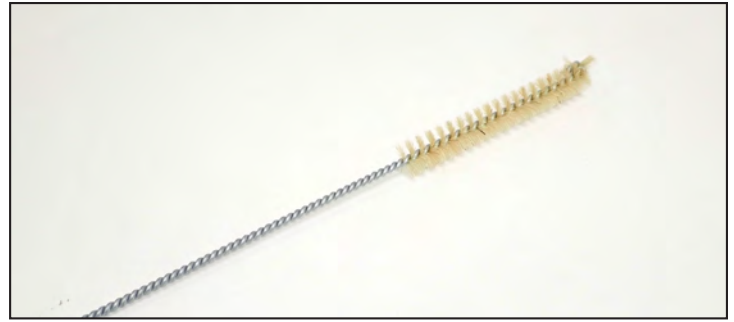
Fig. 1. Narrow tube brush.
