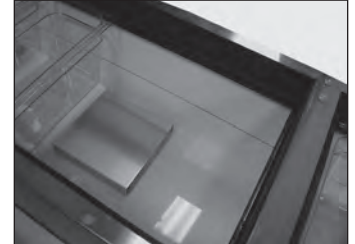
Fig. 2. Correctly positioned baffle.
