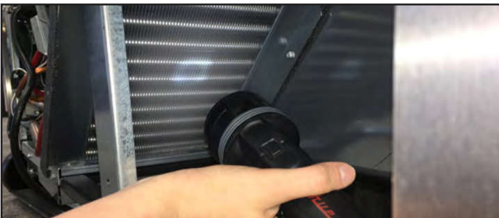
Fig. 4. Verify all blockages have been removed.
