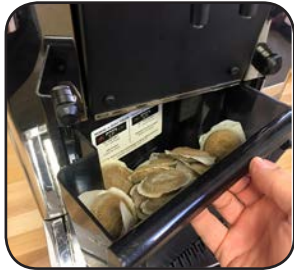
Drawer must be removed for 8 seconds. The counter will automatically re-set after 8 seconds
