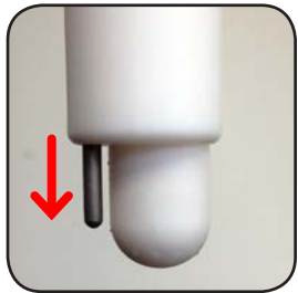
Make sure the probe tip is pushed all the way down when reassembling
