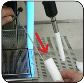
Insert Temperature Probe into outer wand
