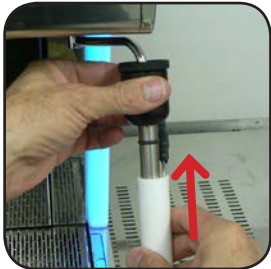
Install Outer wand with probe
