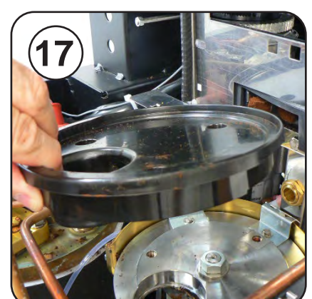
17 Lift Turntable cover off Clean cover with soapy water
