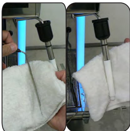
Wipe Temperature Probe and Inner wand
