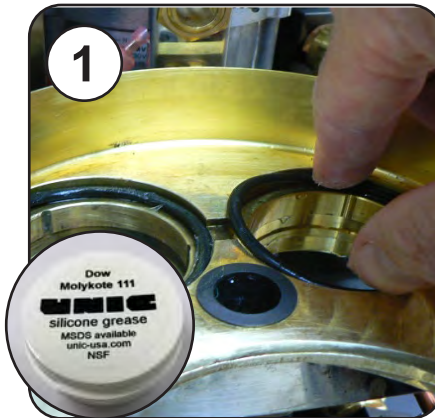
Install new O-rings with Molykote 111 grease
