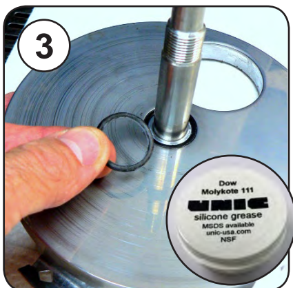
Replace O-ring under Turntable Use Molykote 111
