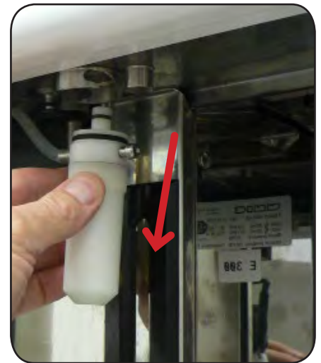
Remove the Foamer by pulling down
