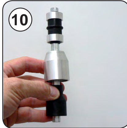
10 Remove Turntable drive shaft
