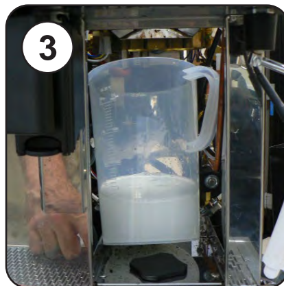
3 For deep cleaning, place a container under the turntable to catch runoff
