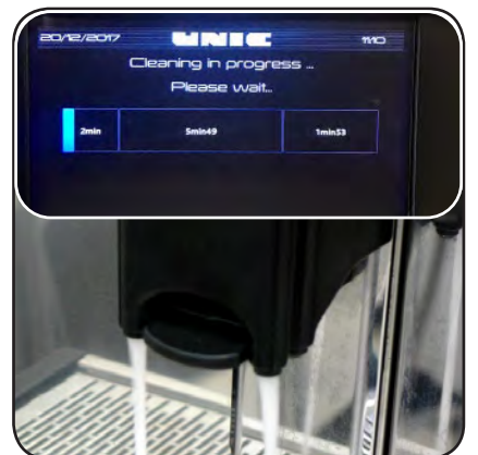
Cleaning Starts Automatically The cycle lasts 10 minutes
