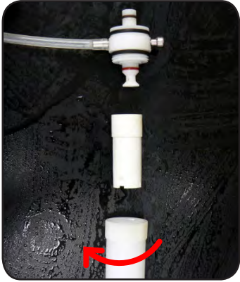
Unscrew the Foamer Cover Tube
