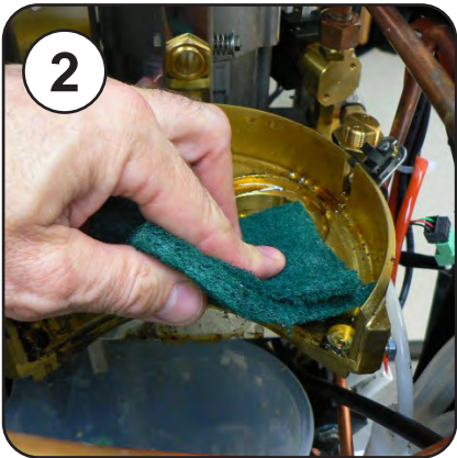
2 Clean the area thoroughly
