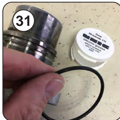
Coat the outer O-ring with Molykote grease
