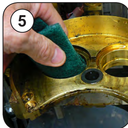
5 Scrub the base with coffee cleaner. Rinse thoroughly.
