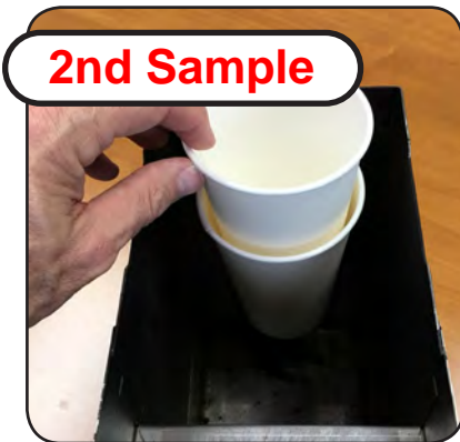
Empty and replace the measuring cup
