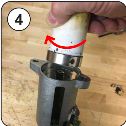
4 Unscrew the inner piston from the jack-screw Left hand threads!
