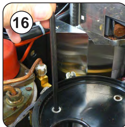
16 Remove the three 6 mm Allen screws from the turntable cover
