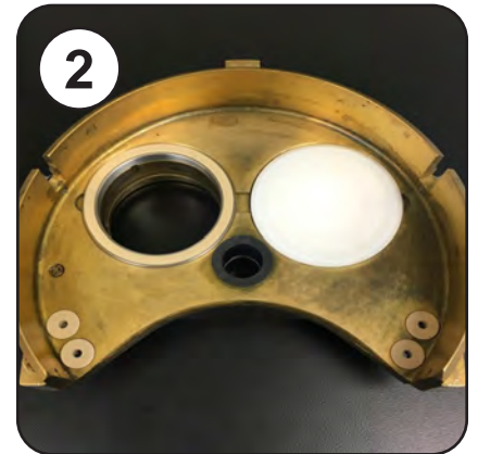
Install seal, 4 support pads, and white plug. No grease!
