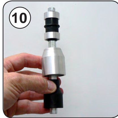
10 Remove Turntable drive-shaft
