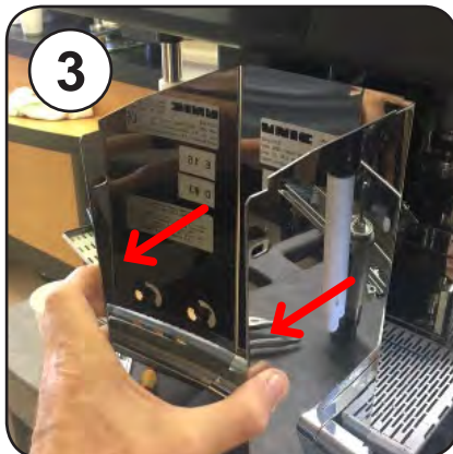
Remove the Inner Panel
