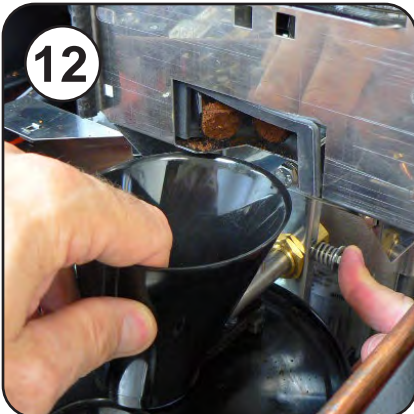
12 Remove Coffee Funnel Press spring latch in while pulling funnel straight out
