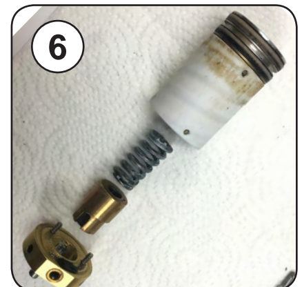
6 Remove the Bottom Plate, Threaded Follower, and Spring
