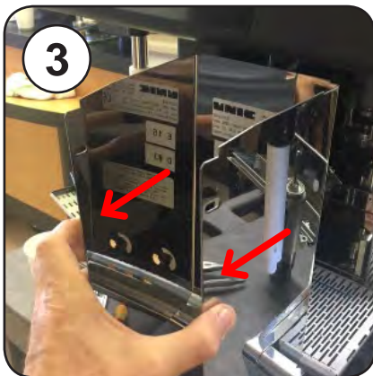
Remove the Inner Panel
