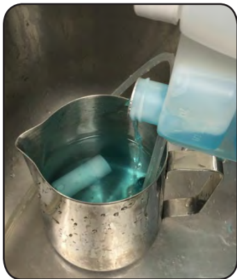
Soak the parts in Rinza solution for 5 minutes
