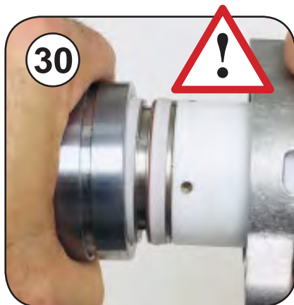
Be very careful not to pinch or roll under the seal edge! (A damaged seal will cause the piston to leak and the Amp draw will be high)
