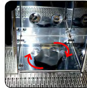
Replace Cleaning Cover Do Not Over-tighten!
