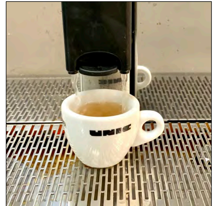
Hopper Sensors can be disabled Water dispenses when hoppers empty
