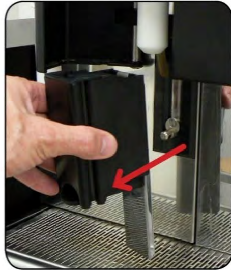
Remove the magnetically mounted spout
