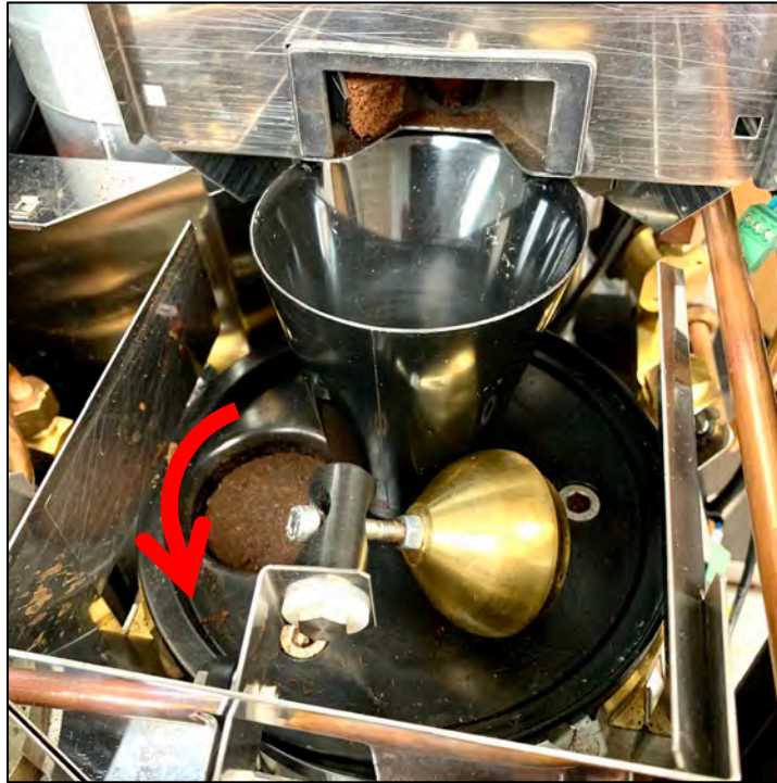
Turntable rotates to Open Position Piston Raises Puck Turntable Rotates to Front
