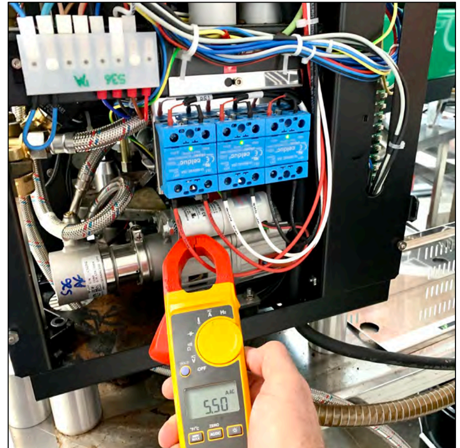
Check for power through all 3 elements More important for older machines
