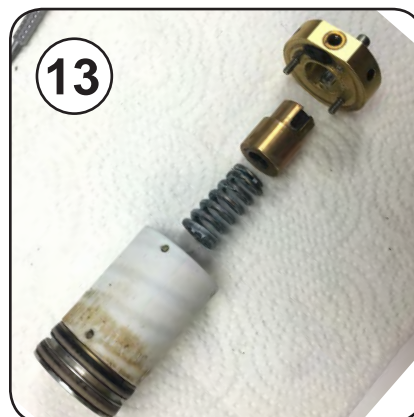
Assemble the spring and lower plate
