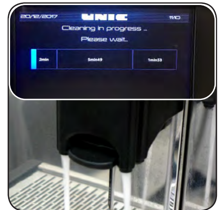
Cleaning Starts Automatically The cycle lasts 10 minutes
