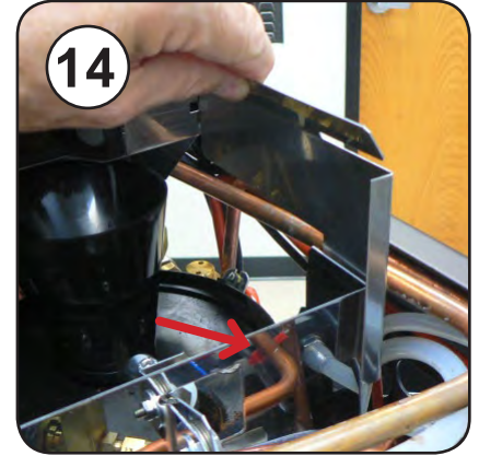
14 Lift both side shrouds straight up
