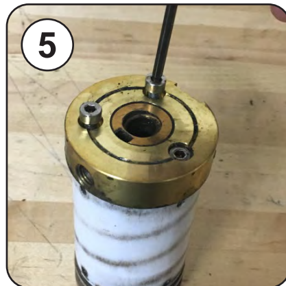
5 Remove the 3 mm Allen screws from the lower plate The spring will decompress!
