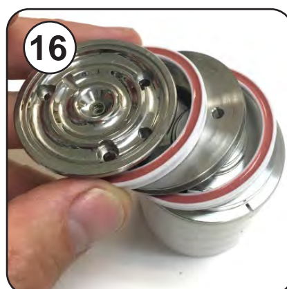
Install the new seals with the orange side up
