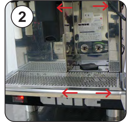
Remove the 4 side screws from the shroud panel
