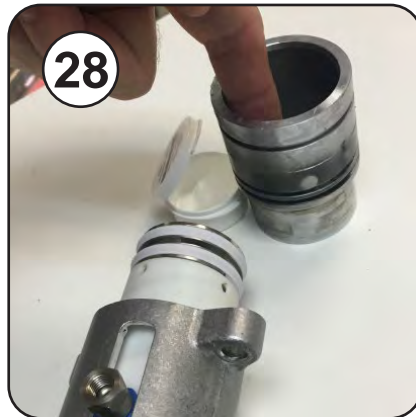
Apply a thin layer of Molykote grease to the brew chamber
