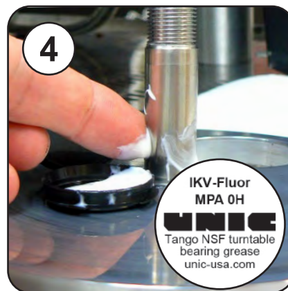
Place a small amount of IKV-Fluor grease on the turntable shaft
