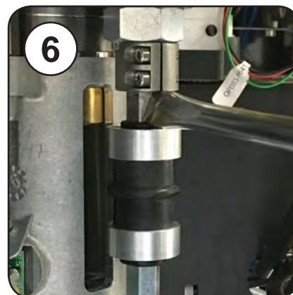
Use a flat screwdriver to push coupling down if necessary
