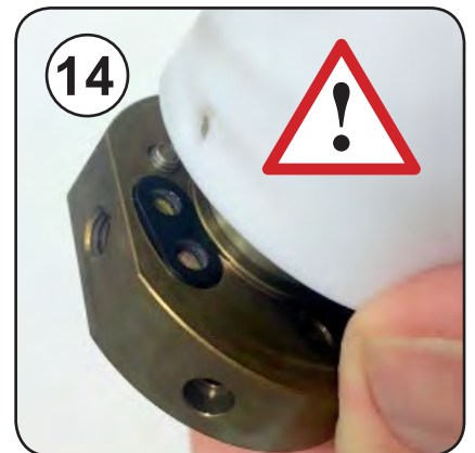
Make sure the holes in the seal line up with the holes in the piston!
