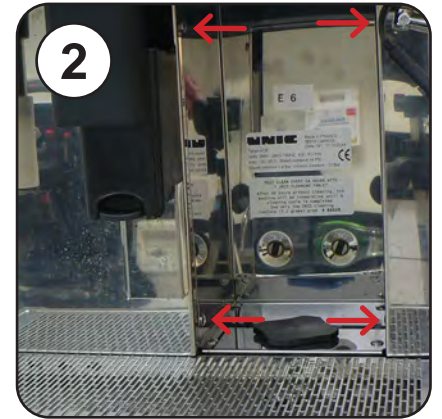
Remove the 4 side screws from the Inner panel
