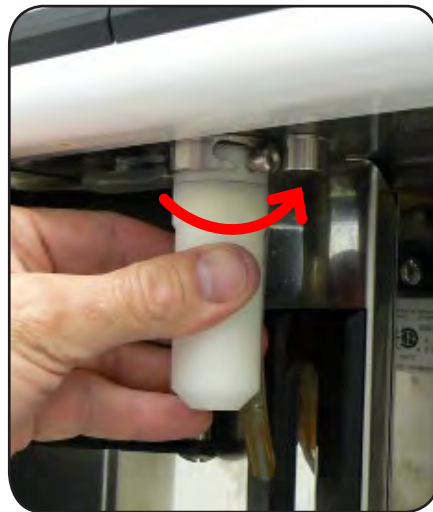
Unlock the Foamer by twisting it to the right
