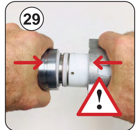
Push the inner piston straight down into the brew chamber
