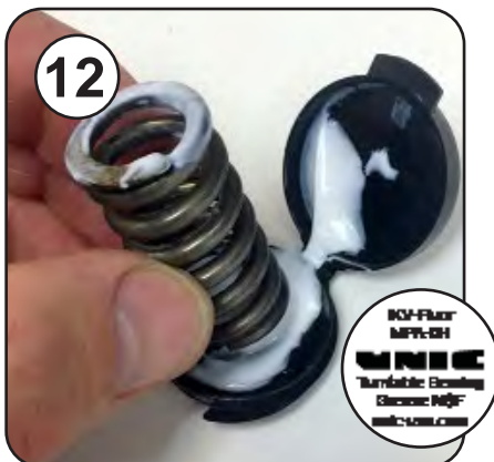
Apply a small amount of IKV-Fluor grease to the ends and SIDES of the spring
