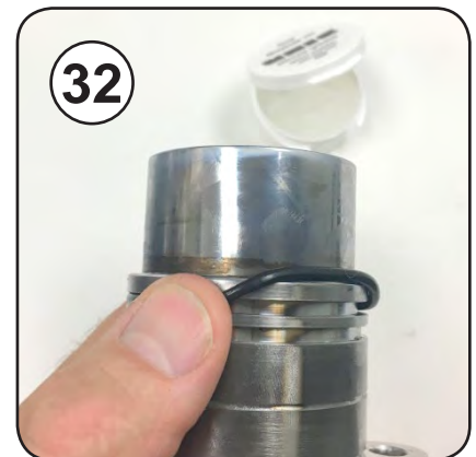
Install the O-ring on the outside of the brew chamber
