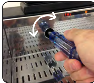
Adjust grinder fine or coarse as needed
