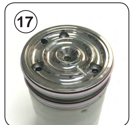
Rotate the pieces until all 4 holds line up
