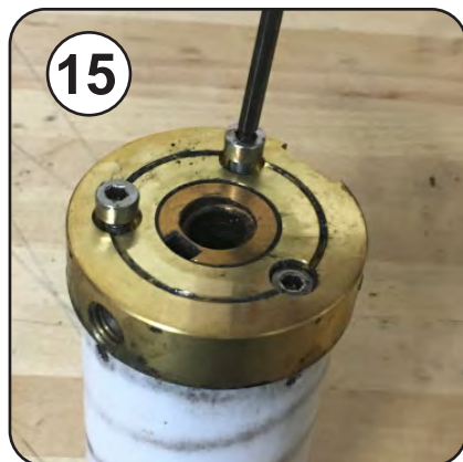
Reinstall the 3 Allen screws The screws will compress the spring; no locktite needed.
