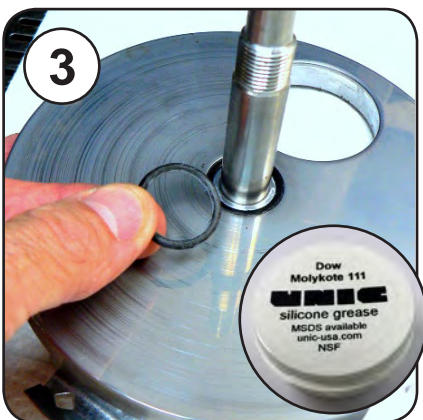
Replace O-ring under Turntable Use Molykote 111
