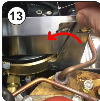
13 Remove side shrouds Loosen 7 mm bolt first Do Not remove bolt
