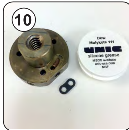
Apply a thin coat of Molykote grease to the new lower seal
