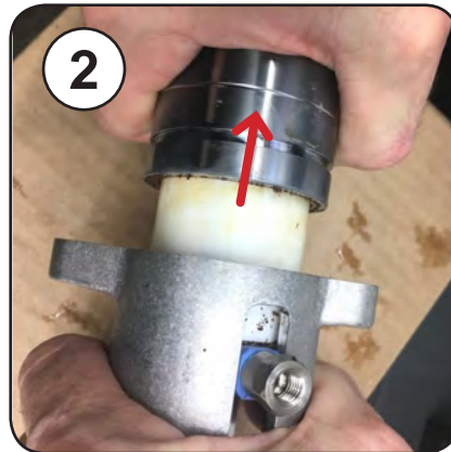
2 Pull the brew chamber off of the piston
