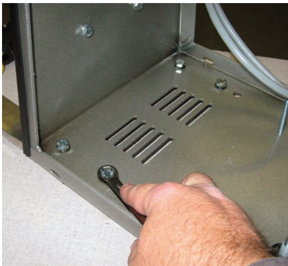
Removal of front feet PM91
