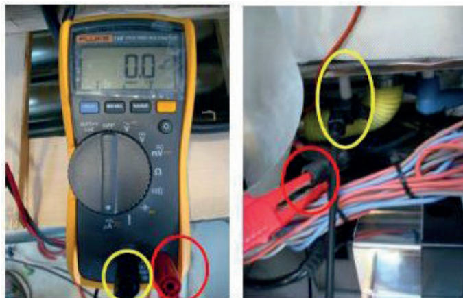
Figure 21 Multimeter connection to the flame control plug
