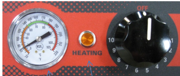
THERMOMETER HEAT INDICATOR LIGHT (Fig.8) THERMOSTAT
