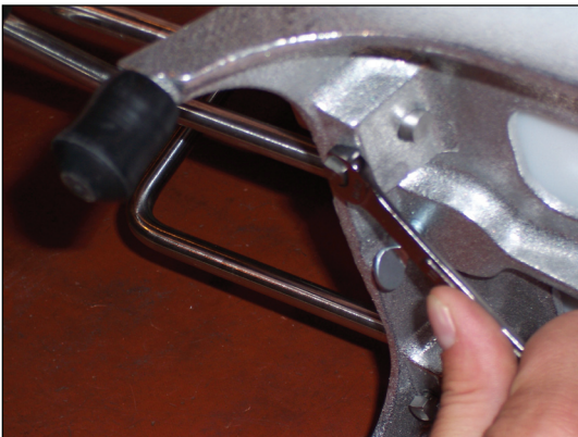
Figure 4. Pusher Head Adjustment Through the Blades.
